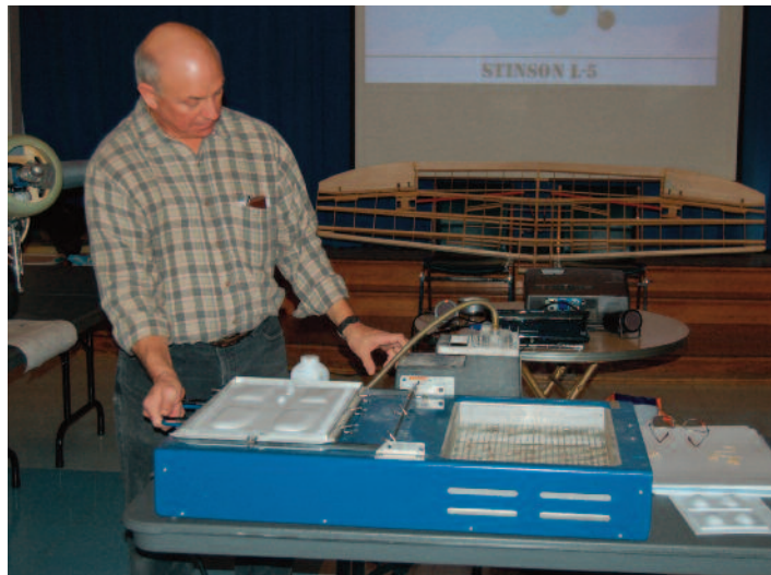
Roy Vaillancourt demonstrating vacuum forming
